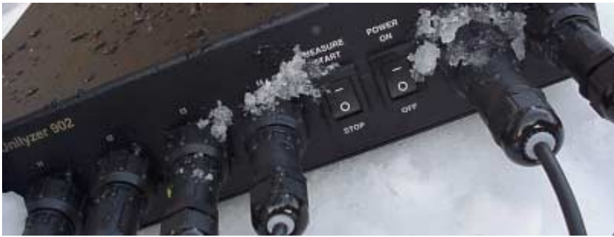
The Unilyzer 902 is dust and splash proof. It can be used in all environments.
